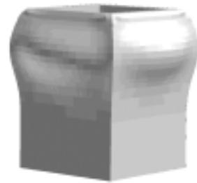
Fig. Deformed shape of a square tube extensional mode ( $L : H = 1 : 2$ )
