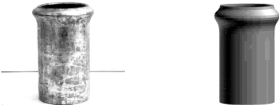
Fig. Deformed shape of a cylindrical tube ( $D : H = 1 : 2$ )
