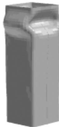
Fig. Deformed shape of a square tube ( $L : H = 1 : 3$ )
