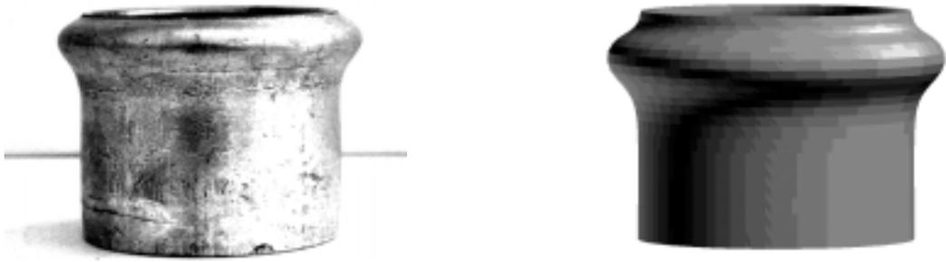
Fig. Deformed shape of a cylindrical tube ( $D : H = 1 : 1$ )
