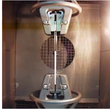
Fig. 2 Tensile test of double-lap joint specimen in environmental chamber
