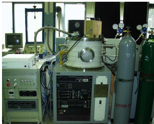
Fig. 1: LEO space environment simulation facility.
