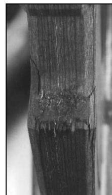
Figure 8 C/C B/D after fracture.
