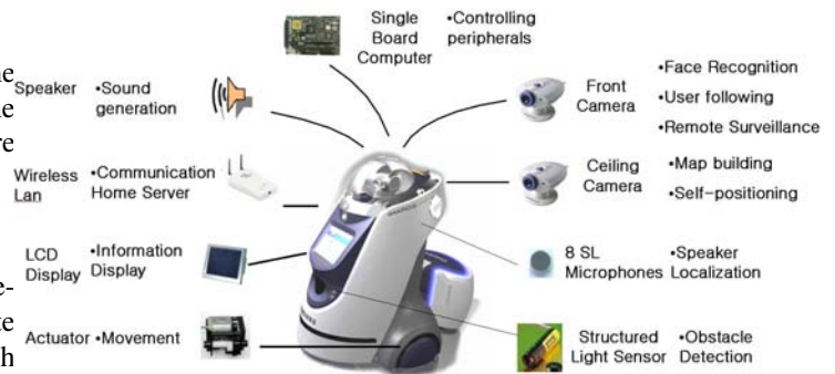
Fig. 1. Components of SHR100
