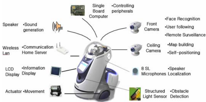
Figure 6. Components of SHR100
