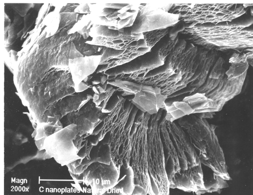
Fig. 5. Partially exfoliated graphite platelets.
