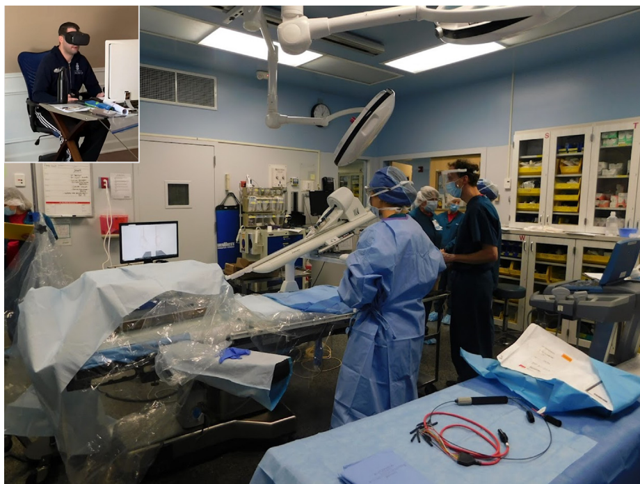
Figure 2 Preclinical telerobotic cardiac catheter ablation in use at Ocean Beach Hospital and Medical Center operating room (Ilwaco, WA) with surgeon in Chicago, Illinois (inset).
