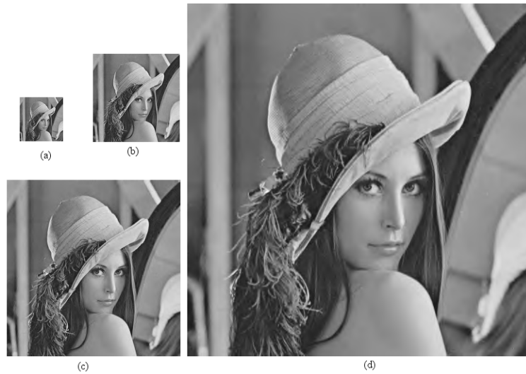
Fig. 4. Reconstructed images with the proposed multiresolutional coding method (bit rate = 1 bpp) from a single bit stream. (a) 1/8 resolution. (b) Quarter resolution. (c) Half resolution. (d) Full resolution.
