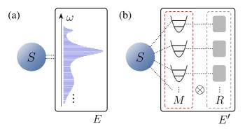
FIG. 1. Schematic diagram showing the two considered models of the system-reservoir interaction. (a) An OQS S interacting with a bosonic environment E. (b) The same system S interacting with an auxiliary environment E', consisting of a finite number of discrete modes M coupled to local Markovian reservoirs R.
