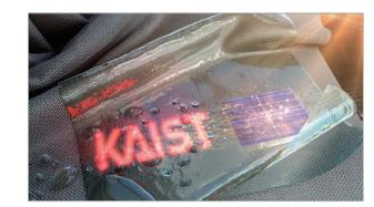
To this end, a new encapsulation technique was developed in which a flexible silica polymer solution and a nano-stratified structure made of aluminum oxide (Al203) and zinc oxide (Zn0) were laminated. Improvement of washing characteristics through protonation-deprotonation reaction was confirmed through Fourier-transform infrared spectroscopy (FT-IR), water vapor transmission rate (WVTR), and surface roughness change analyses.
