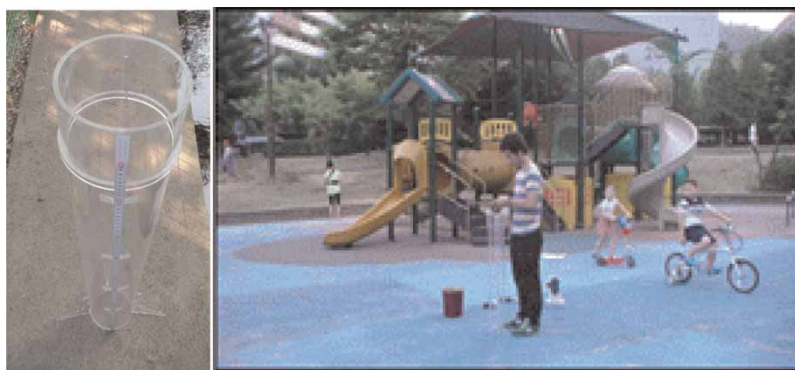
Figure 1 | Equipment for measuring coefficient of restitution and measuring coefficient of restitution.
