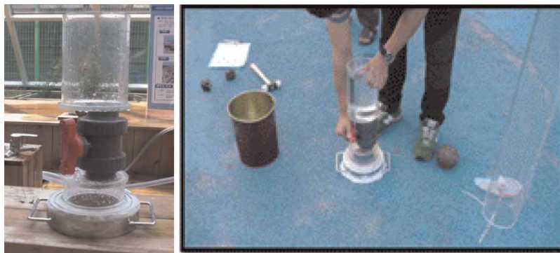
Figure 2 | Equipment for measuring permeability and measuring permeability of UESF.
