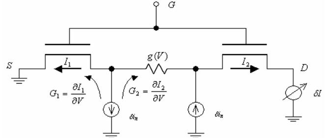
Fig.1. Impedance Field Method
