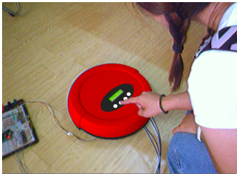
Fig. 4 Appearance and interface test of a cleaning robot
