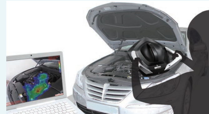
(Figure 2) Identifying the location of target noises by using SeeSV-S205, a portable sound camera.
