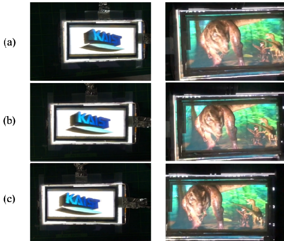
Fig. 16. Parallax motion of the 3D images viewed at (a) -18^\circ (b) 0^\circ (c) 18^\circ from the display.
