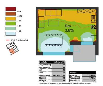
Figure 1: Example of graphical translation of results from a daylight and energy-balance simulation program. Seventh semester student project. The representations explain the changes caused by altering the design of the balcony.
