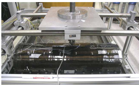
Fig. 4 Experimental setup of the quasi-static loading test.
