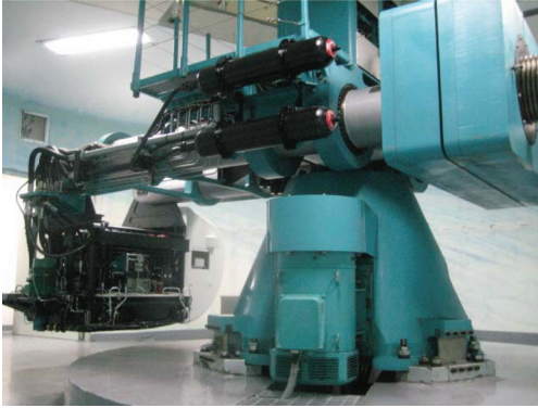
Figure 1. KAIST geo-centrifuge with earthquake simulator.
