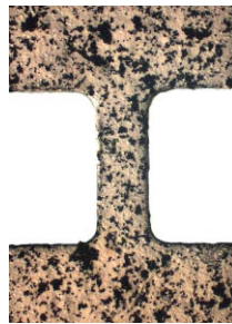
Figure 4. Speckle pattern generated on the surface of the micro specimen using toner powder.
