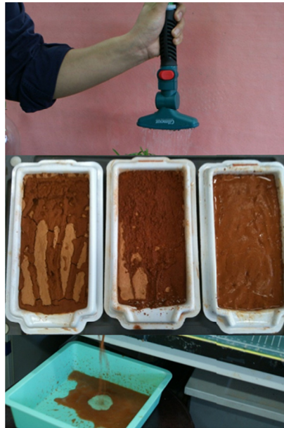
FIG. 2. Laboratory precipitation simulation of soils to evaluate the erosion resistance of biopolymer treated soils.
