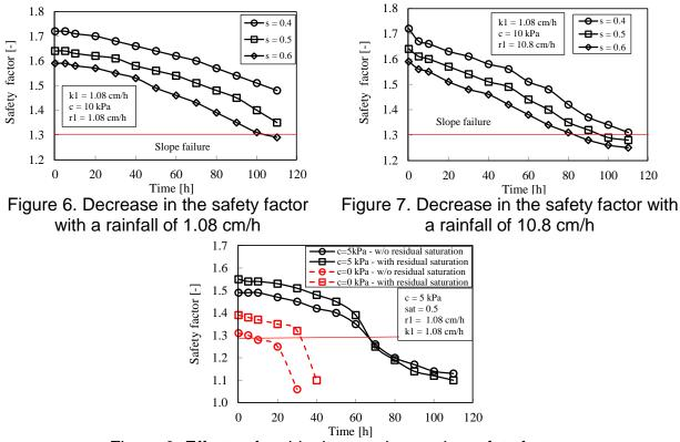
Figure 8. Effects of residual saturation on the safety factor
