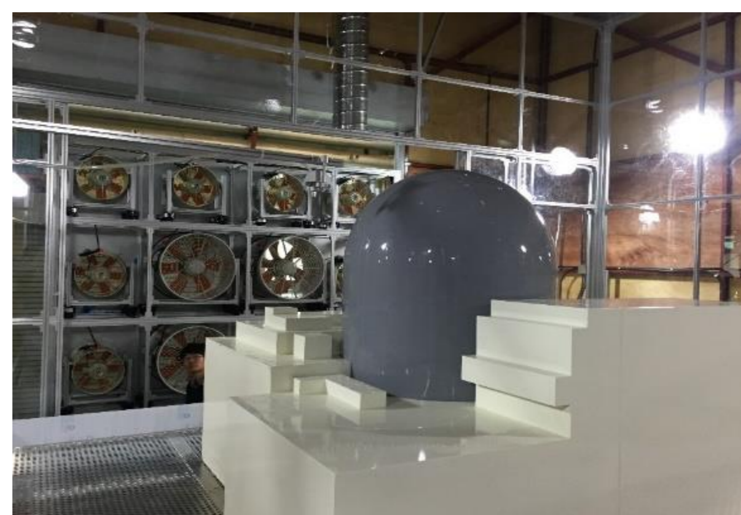
Fig. 2. Scaled down (1 : 50) NPP model
