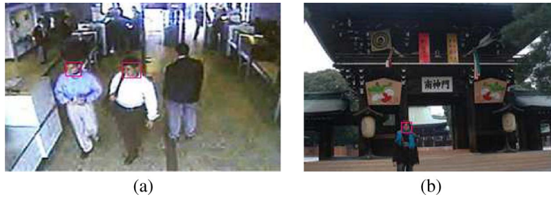
Fig. 1. Practical illustrations of extremely small-sized faces in FR-based applications. (a) Surveillance video frame from “Washington Dulles International Airport.” The two face regions occupy approximately 18 \times 18 pixels of the video frame shown, having an original resolution of 410 \times 258 pixels. (b) Personal photo from a “Flickr” [19] web site. The face region occupies about 14 \times 14 pixels in the picture shown, having an original resolution of 500 \times 333 pixels.
