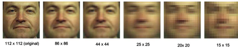
Fig. 4. Examples of facial images from color FERET according to six different face resolutions. A low-resolution observation below the original 112 \times 112 pixels is interpolated using nearest-neighbor interpolation.
