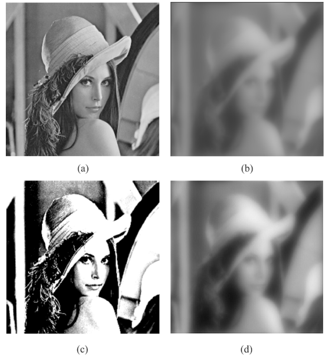
Fig. 10. Adaptation (contrast stretching) for the "loss of fine detail" symptom: (a) original image; (b) simulated image with L_d = 0.9 ; (c) adapted image; and (d) simulated image ( L_d = 0.9 ) of adapted image (c).
