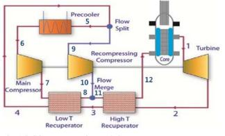
Fig. 1 S-CO<sub>2</sub> recompressing cycle layout
