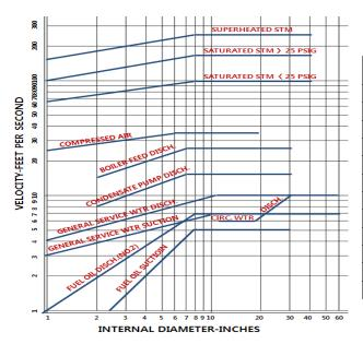
Fig. 2 The optimal flow velocity of various piping systems [4]
