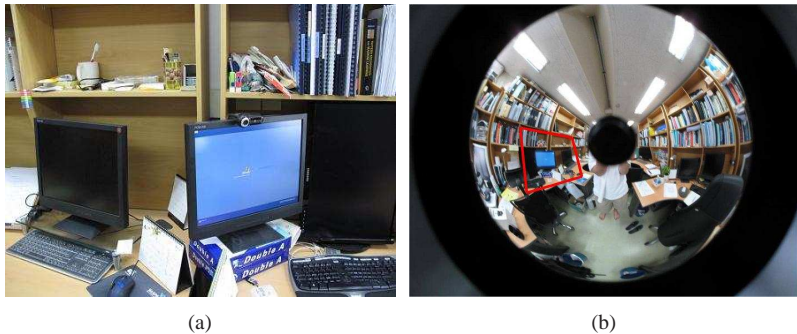
Figure 1: Compared to a traditional perspective camera (left), a catadioptric system (right) can gather much more information from the environment thanks to its wide field of view. These two images have been acquired at the same position. The red box (in the right image) corresponds to the portion of the perspective image included in the catadioptric image. In the following, we will refer to the blind spot at the image center as the “inner circle” and the large circular boundary as the “outer” circle.
