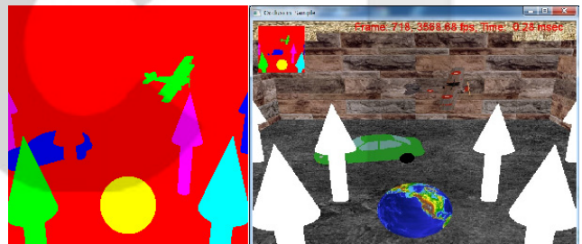
Fig. 8. Results of occlusion computation (left, occlusion map image; right, screen image of sample run).
