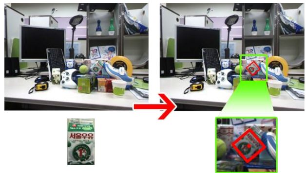
Fig. 1: Left input image is captured by our intelligent robot. When the robot asked to detect milk pack (though milk is small in input image), utilizing our approach (right image) shows appropriate object detection result - the correct location and orientation.
