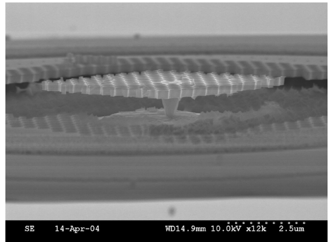
Fig. 4. Cross-sectional SEM image. Dusts around the post are remnants of the PR produced in the intentional breaking process.
