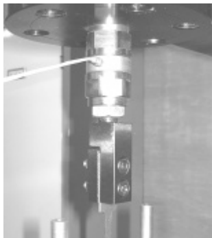
Fig. 2 Load cell and an upper jig
