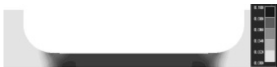
Fig. 5 Contour of the effective plastic strain of a specimen with the gauge length of 30 mm at strain of 0.2
