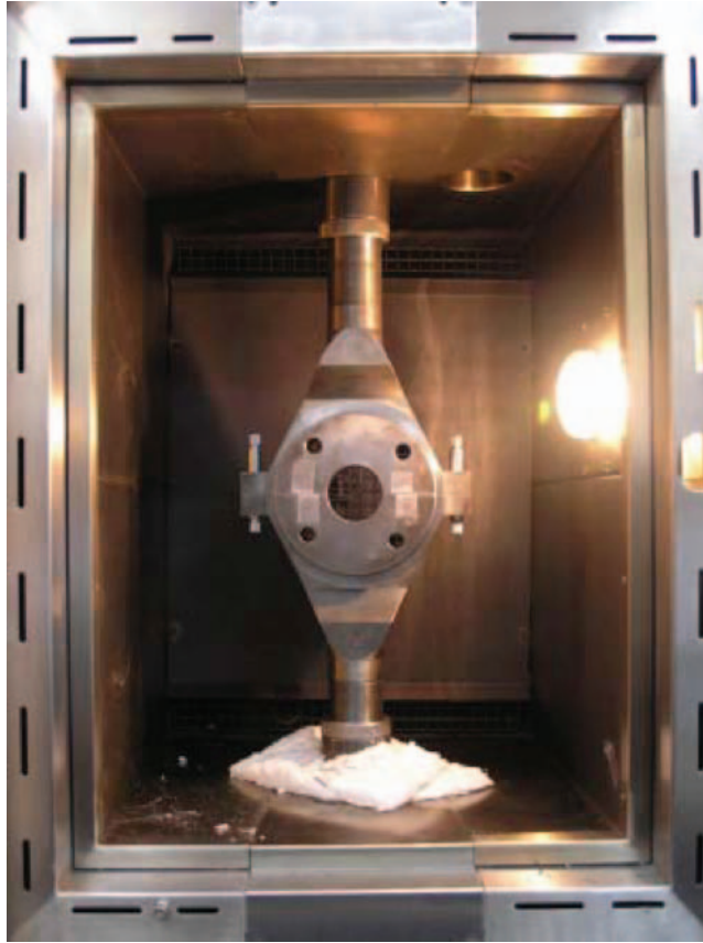
Figure 7. Experimental setup for the composite/aluminum ring specimen under cryogenic environment.
