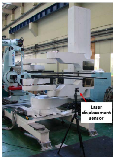
Figure 7. Experimental setup to measure the fork end vibration after P1 axis motion
