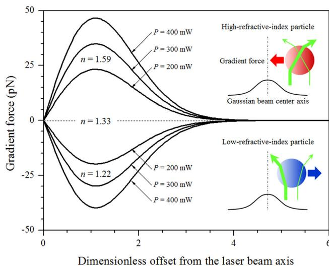
FIG. 2. The gradient force acting on PSL (high-refractive-index) and hollow glass (low-refractive-index) particles under various laser beam powers. The inset illustrates the principles underlying the positive and negative gradient forces.
