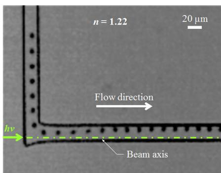
FIG. 4. Trajectories of a hollow glass (low-refractive-index) particle (enhanced online) [URL: <http://dx.doi.org/10.1063/1.4817938.2>].
