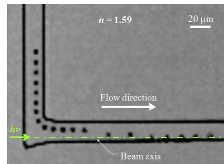
FIG. 3. Trajectories of a PSL (high-refractive-index) particle (enhanced online) [URL: <http://dx.doi.org/10.1063/1.4817938.1>].
