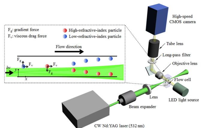
FIG. 1. Schematic diagram of the experimental setup. The laser wavelength was 532 nm. The inset shows the principle underlying the present optofluidic particle manipulation system. The laser beam center axis was aligned adjacent and parallel to the sidewall of the microfluidic channel.
