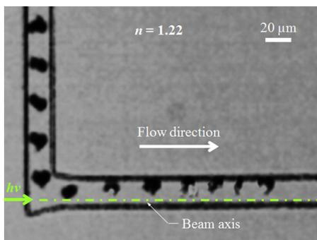
FIG. 5. Trajectories of the doubly attached hollow glass particles (enhanced online) [URL: <http://dx.doi.org/10.1063/1.4817938.3>].
