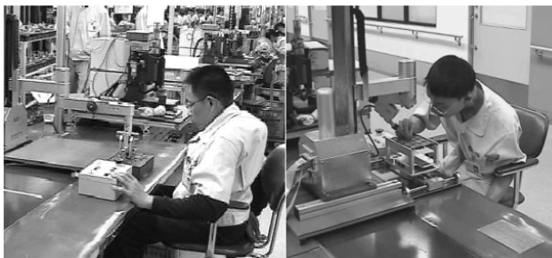
Fig. 11. Field test: 1. Test work on the circuit of PCB, 2. Soldering inspection and repairing work on PCB
