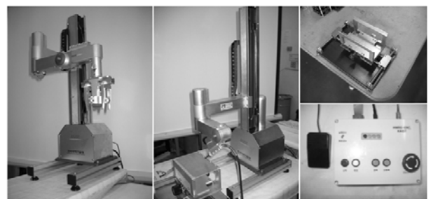
Fig. 10. Developed robot arm, XY table and Interface device. the left figure indicates the initial position of robot for Circuit test of PCB ; and middle figure indicates the initial position of robot for Soldering inspection and repairing of PCB . And the right top figure indicates XY table used for the user to find a position for repairs.
