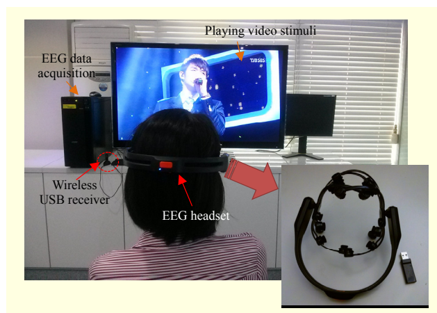
Fig. 3. Experimental environment. While subjects wearing EEG headset view their personalized video stimuli, raw EEG data from EEG headset is accumulated through wireless transmission.
