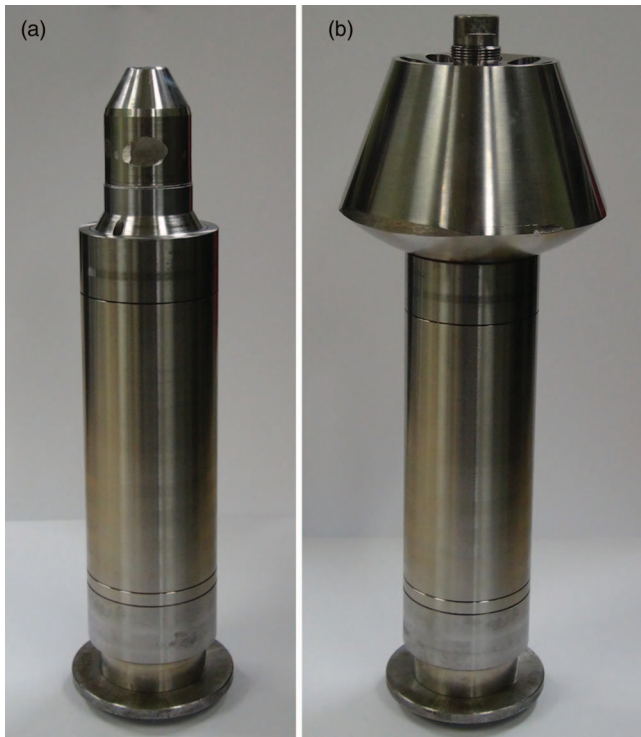
FIG. 5. Fabricated rotor-shaft. (a) Shaft only; (b) Rotor-shaft assembly.
