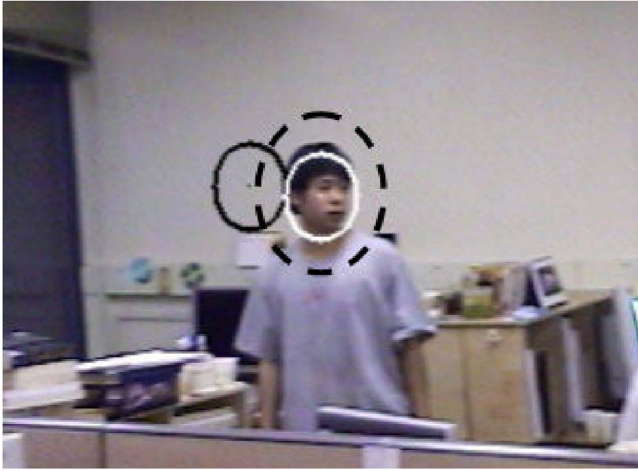
Fig. 4 Initial position for mean shift that is adjusted by the background motion compensation in frame 294 of the Walking sequence. Black and white ellipses represent the initial position obtained before and after background motion compensation, respectively. The black ellipse resides outside the ROC, described by a dashed line.
