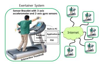
Figure 1. Architecture of the system
