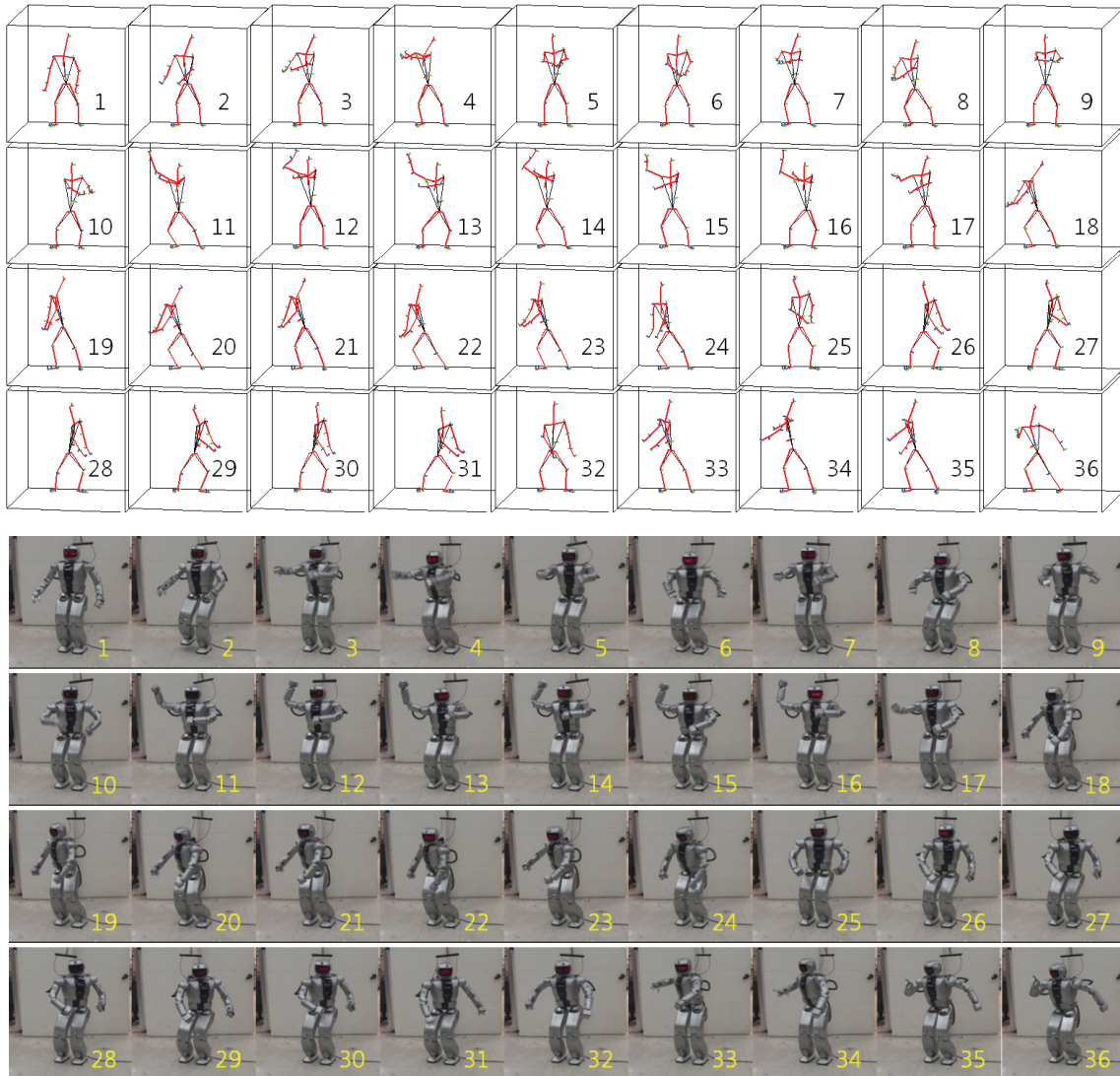
Figure 21. Captured human motion and imitated motion by a humanoid robot in Experiment 5.3.
