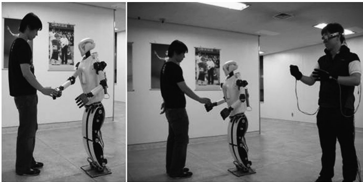
Figure 8. Object grasping and delivery experiment.
