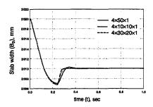
Figure 5. The transient response of neural network controller
