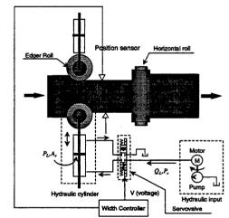
Figure 2. The structure of the automtic width control system
