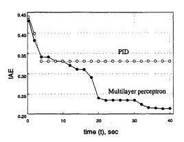
Figure 8. The integral absolute errors
