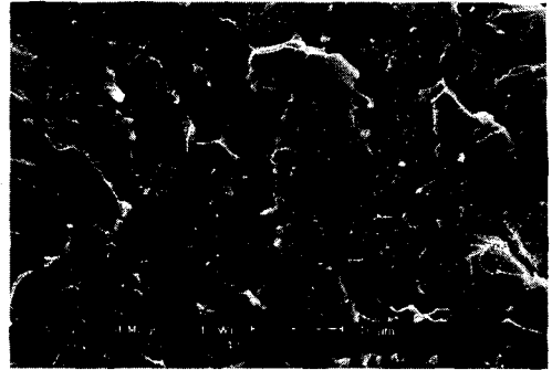
Fig. 5 A SEM image of a fractured surface of 1.0 wt% MWNT/epoxy composites.
