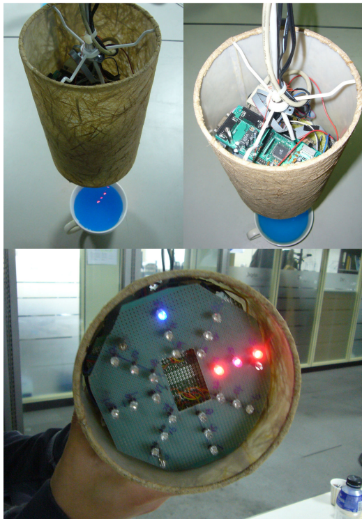
Fig 4: The hardware structure of Tea Place: Reflected image on the surface of Poweraid drink (top left), Electric core unit (top right), LED array (bottom)
