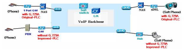
Fig. 7. Configuration of simulation environment applying proposed QoS-factor scheme and improved PLC algorithm
