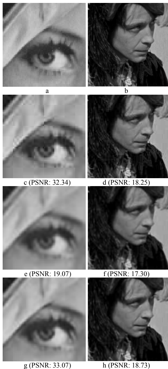
Fig. 3. Enlarged portions of image reconstructions: a and b. original images, c and d. JPEG encoded images, e and f. smoothed images, and g and h. results obtained with proposed method.
