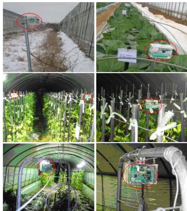
Figure 4. A-node (top-leftmost) in the outside of the greenhouse. A-nodes (red-circled ones) deployed in greenhouses with cabbage (top-leftmost) and melon
