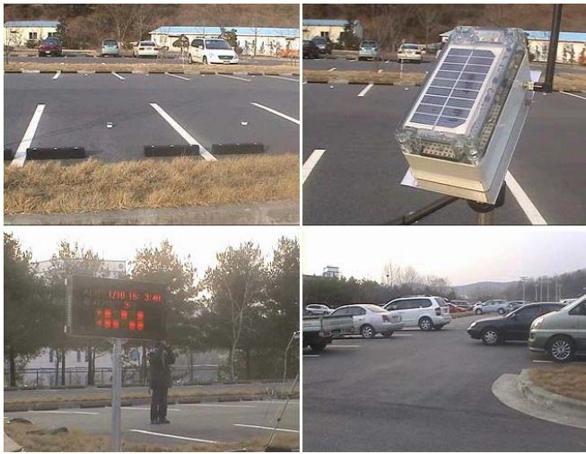
Figure 9. Demonstration of PGS system. 1) T-Sensor nodes in parking lots, 2) T-Sink Node, 3) 7 cars in the parking lots, and 4) VMS which is displaying the available parking lots (from left-top to left-bottom in clock-wise direction)
