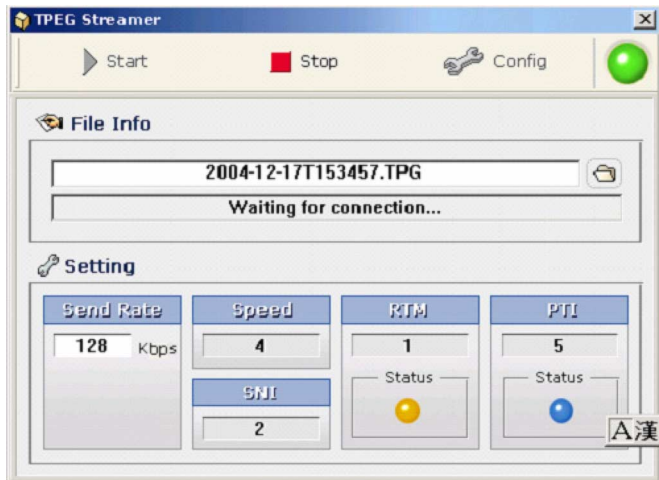
Fig. 5. Stream server user interface. It includes the start and stop button for the beginning of the streaming with the specified stream rate and configuration button for the connection with the ensemble multiplex or data server. It also has several connection status monitoring displays.
