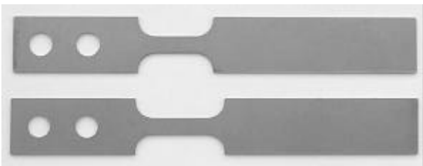
Fig. 4 Tensile specimens with the length of the gauge section of 15 mm and 20 mm.
